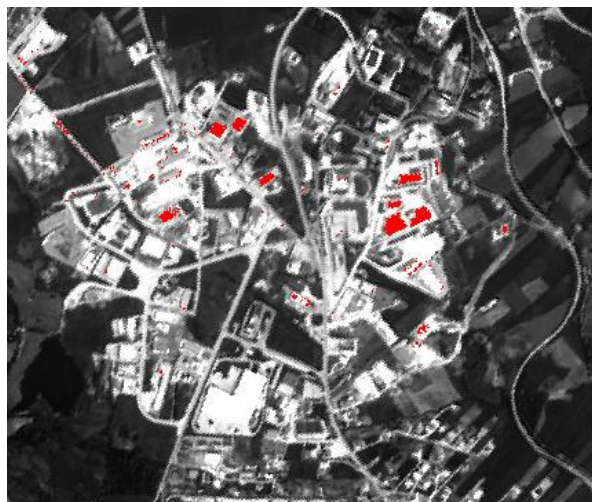
Fig 4 Coperture in C-A in area industriale
