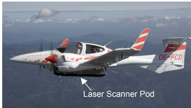
Fig.3 Laser Scanner Pod mounted under the DA42-MPP's fuselage
